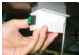
Push button switch box
