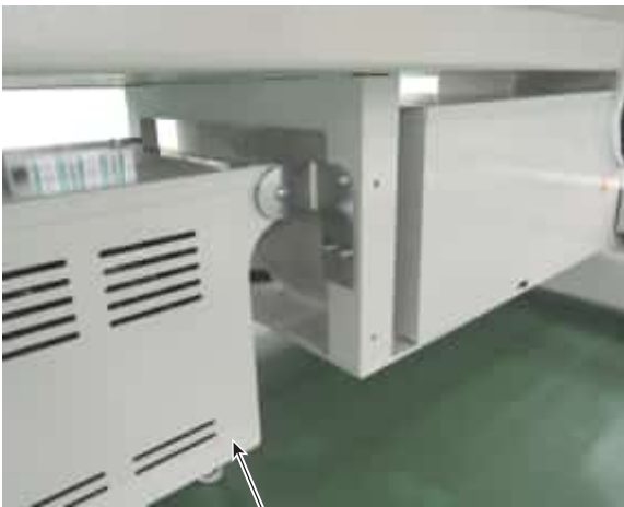
Extension device controller
