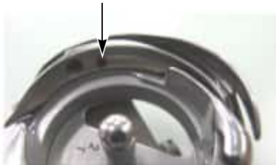
Lubrication hole (red mark)
