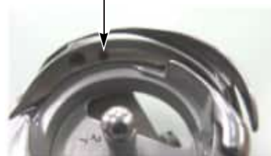
Lubrication hole (red mark)
