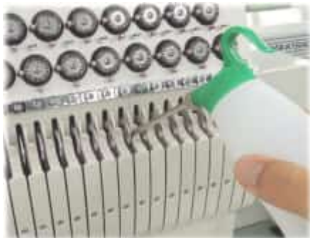
Needle bar (upper part) A in the right figure
